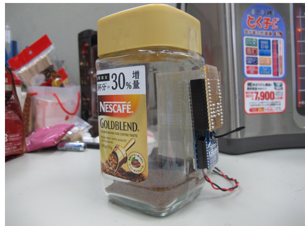
(b) The “Coffee Container” with gyro sensor
