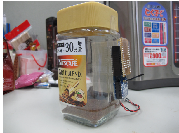
(b) The “Coffee Container” with gyro sensor
