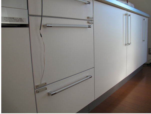
Figure 4.6: The “Cupboard” with magnetic sensor
