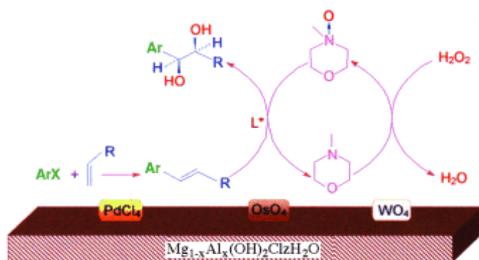
Scheme 7 The catalytic cycle in the LDH-PdOsW-catalyzed synthesis of chiral diols using \text{H}_2\text{O}_2 as the terminal oxidant. [Reproduced with permission from Wiley-VCH of ref. 136]
