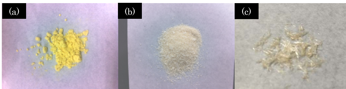
Figure 2.1 The physical appearance of (a) 4ACA (b) the crude of 4,4'-diamino- \alpha -truxillic acid dihydrochloride and (c) the crystal of 4,4'-diamino- \alpha -truxillic acid dihydrochloride.
