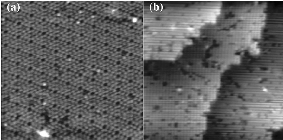
Figure 6 STM images taken with W tips fabricated using the liquid metal electrode. (a) STM image of a Si(111)-7×7 surface; scanning area: about 18 nm to 27 nm, tunneling current: 0.05 nA, tip voltage: -1.5 V. (b) Si(001)-2×1 surface; scanning area: about 36 nm to 38 nm; tunneling current: 0.1 nA, tip voltage: 1.5 V.
