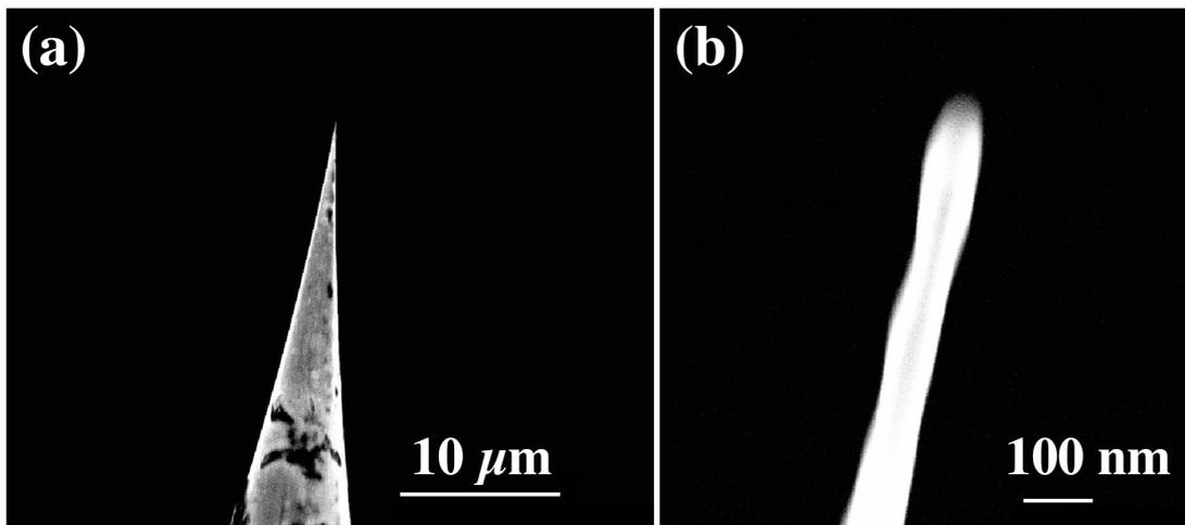
Figure 4 (a) SEM image of a W tip fabricated in the procedure using the liquid metal electrode.
