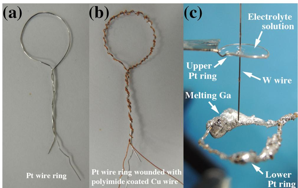
Figure 3 (a) Pt wire ring, (b) Pt wire of the ring is wound with a polyimide-coated Cu fine wire of 0.15 mm in diameter as a heater, and (c) photo of the setup with a Pt ring (upper) and a Pt ring wound the Cu wire (lower) covered with liquid metal Ga.
