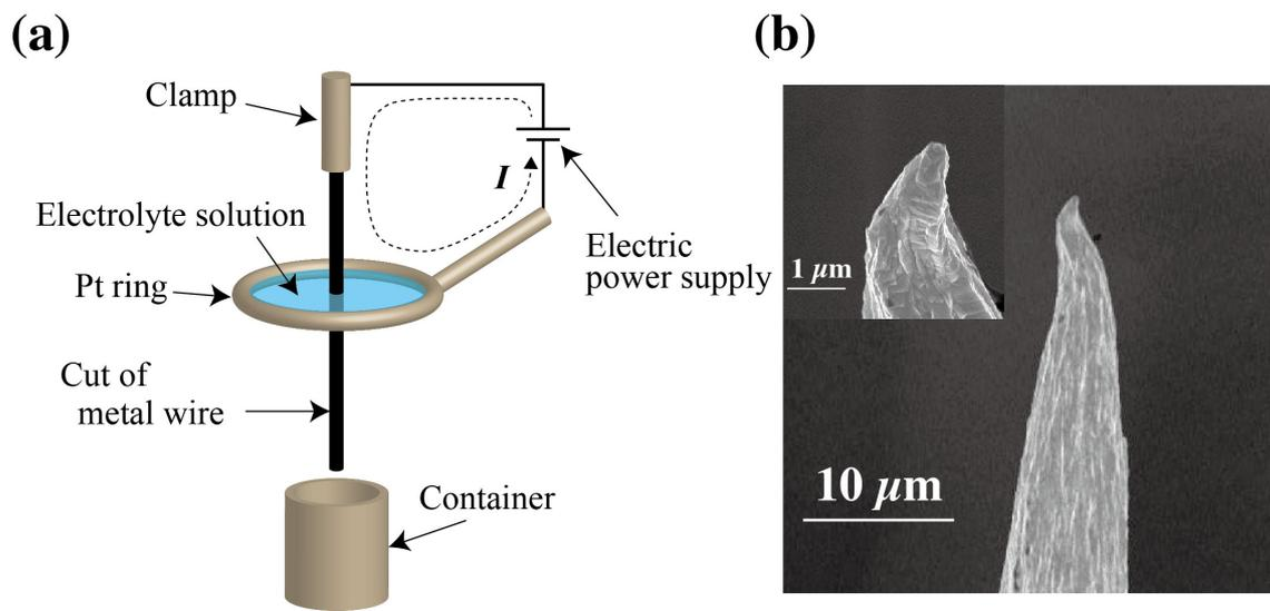
Figure 1 (a) Schematic of a typical setup to fabricate STM tips by electrochemical etching in a meniscus solution in a Pt ring. (b) SEM image of a bent tip of polycrystalline W wire prepared using this setup, as an example. Inset shows a magnified image of the tip.
