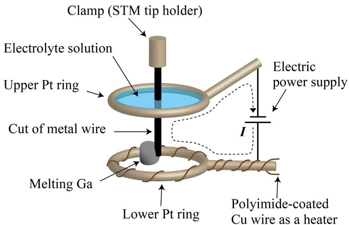
Figure 2 Schematic of the setup of electrochemical etching with a liquid metal electrode.
