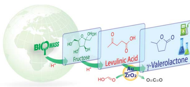
Figure 2. Dehydration/hydrogenation of biomass-derived compounds to \gamma -valerolactone
