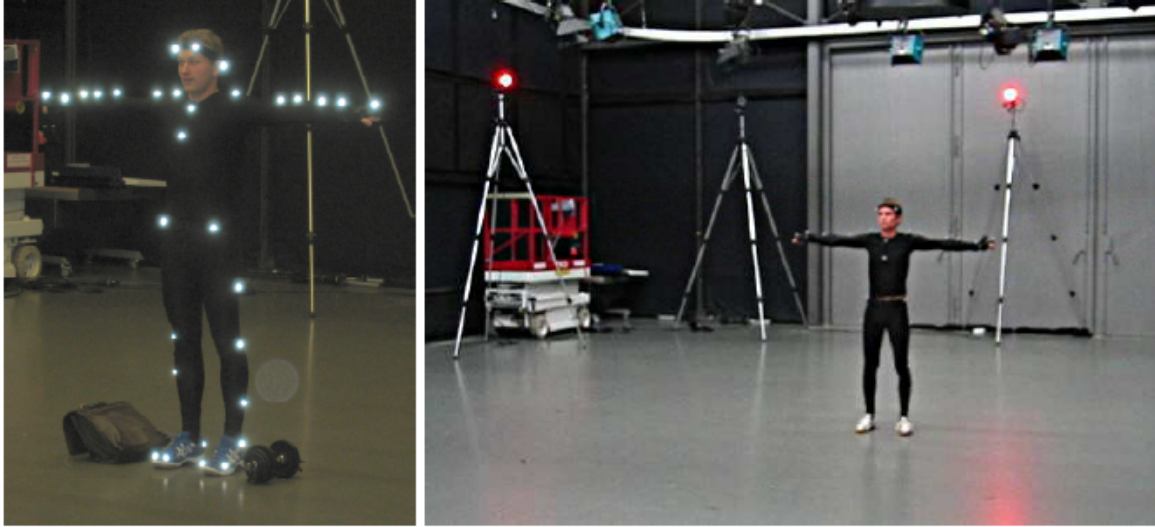
Figure 2.1: Passive optical motion capture system based on retro-reflective markers attached to the actor’s body [25].
