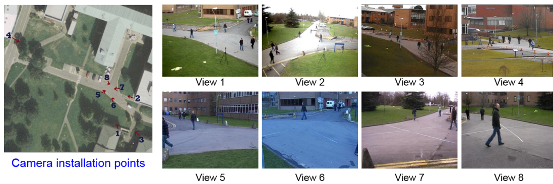
Figure 6.1: A surveillance system monitors the presence of visitors in a university campus. It uses eight cameras installed at different location (the leftmost figure) to capture information at multiple viewpoints (View 1-8). Images are obtained from the PETS 2009 dataset [6].
