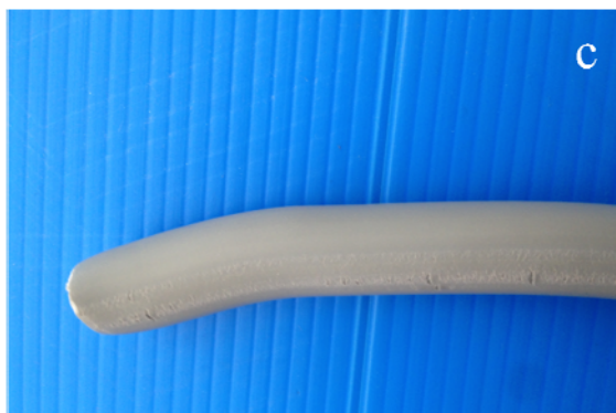
Figure 6 Pictures of surface of PVC samples: a. sample 4 (PVC, 900 rpm, T_{\text{aver.}} = 180.4\text{ }^{\circ}\text{C} ), b. sample 5 (PVC, 900 rpm, T_{\text{aver.}} = 191.6\text{ }^{\circ}\text{C} ) and c. sample 6 (PVC, 450 rpm, T_{\text{aver.}} = 191.6\text{ }^{\circ}\text{C} )
