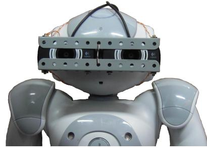
Fig. 4. Aldebaran Nao humanoid robot with mounted cameras.
