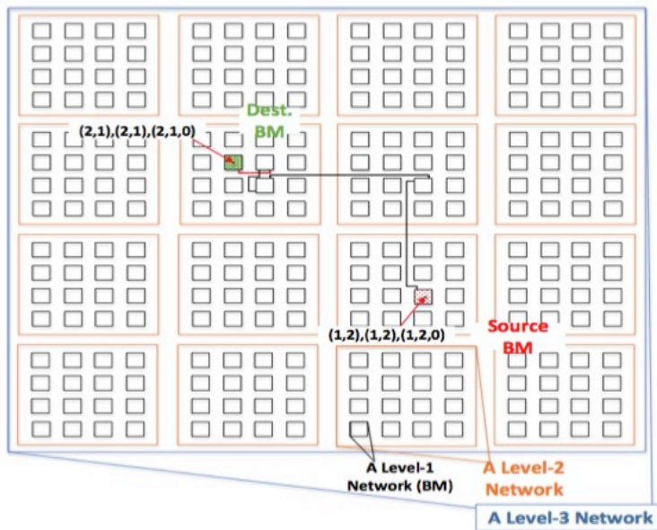
Figure 3.4: Routing Path for 3D-TESH Network
