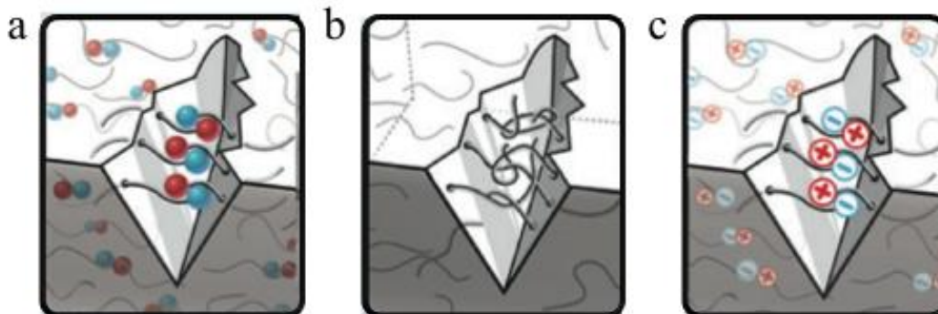
Figure 3-5 Illustration of intrinsic self-healing materials 39 (a) Reversible bonding, (b) Molecular interdiffusion and (c) Ionomeric self-healing (Blaiszik, B., Macromolecules , 2010)
