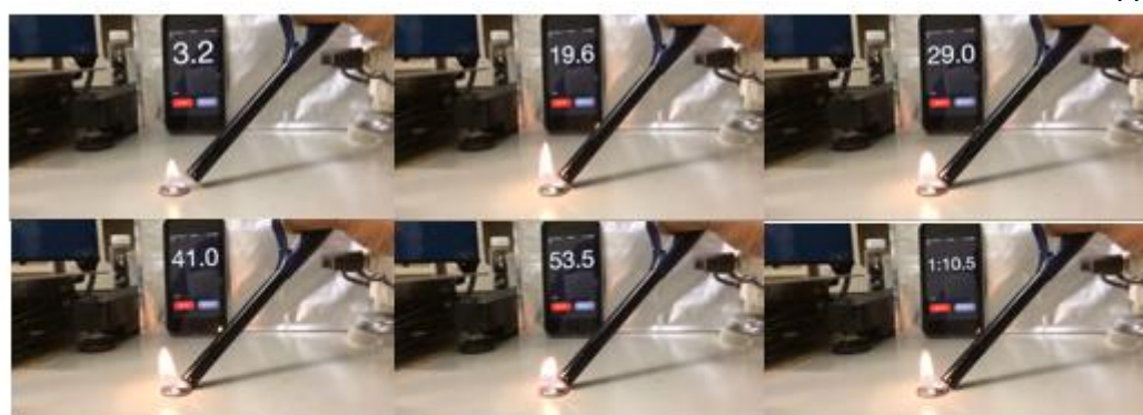
Time-sequenced flammability studies of Hybrid E
