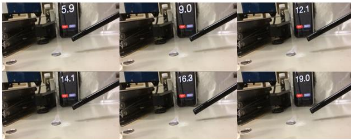
Figure 4.19 Flammability studies of 1MLiPF 6 (1:1 EC-DEC) solution
