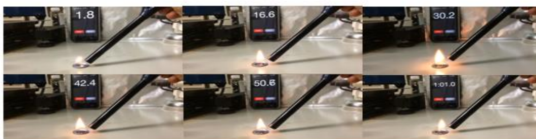
Time-sequenced flammability studies of Hybrid H
