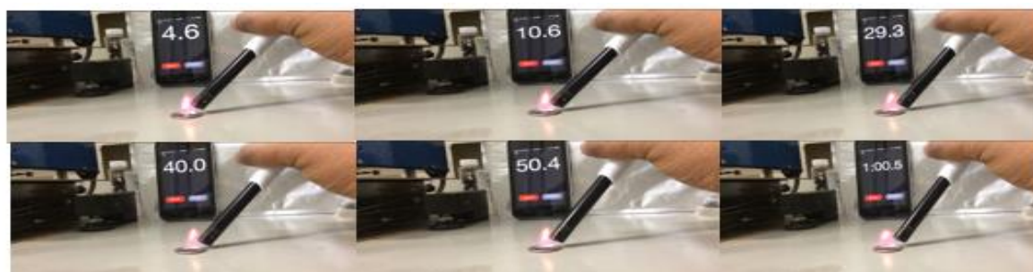
Time-sequenced flammability studies of Hybrid C
