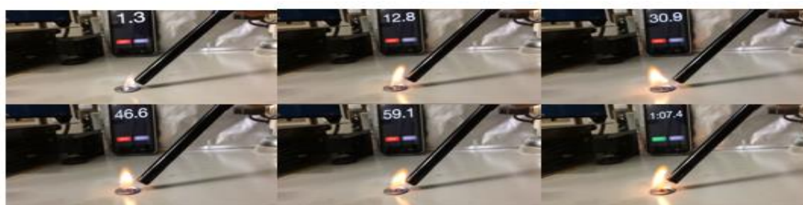
Time-sequenced flammability studies of Hybrid I
