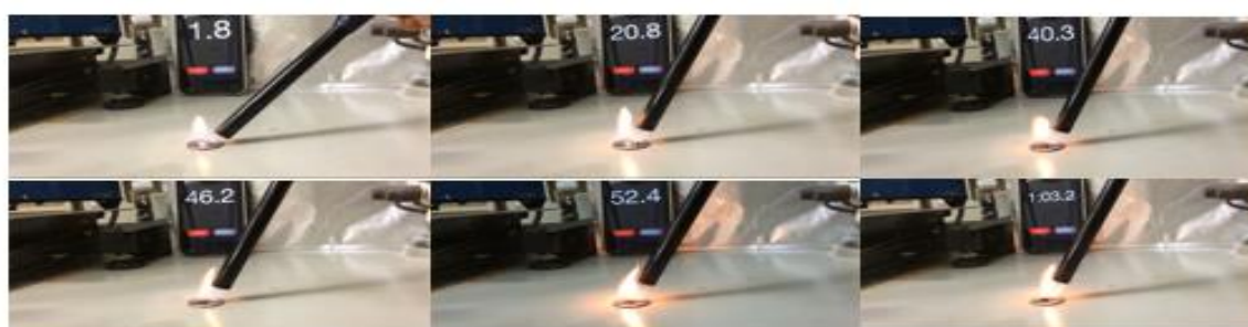
Time-sequenced flammability studies of Hybrid K
