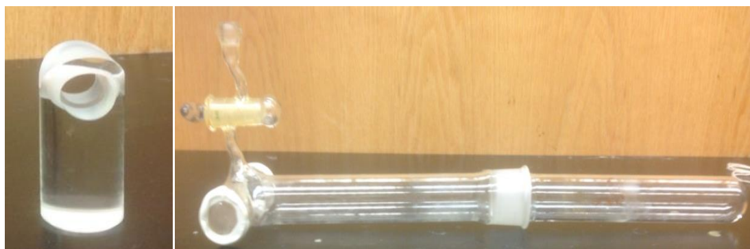
Figure 1. Pellet holder (left), Reactor for IR, activation and ethylene oligomerization (right)
