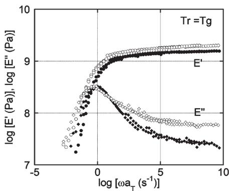
Fig. 5. Master curves of (circles) tensile storage modulus  $E'$  and (diamonds) loss modulus  $E''$  for (closed symbols) PC and (open symbols) PC/ $p$ -tPh (10 wt%). The reference temperature is  $T_g$  determined by DSC measurements.
