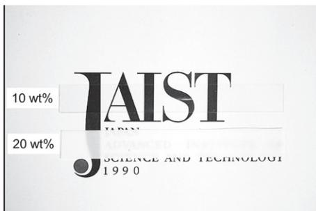
Fig. 2. Sample specimens with 300  $\mu\text{m}$  thickness; (top) 10 wt% and (bottom) 20 wt% of *p*-tPh.
