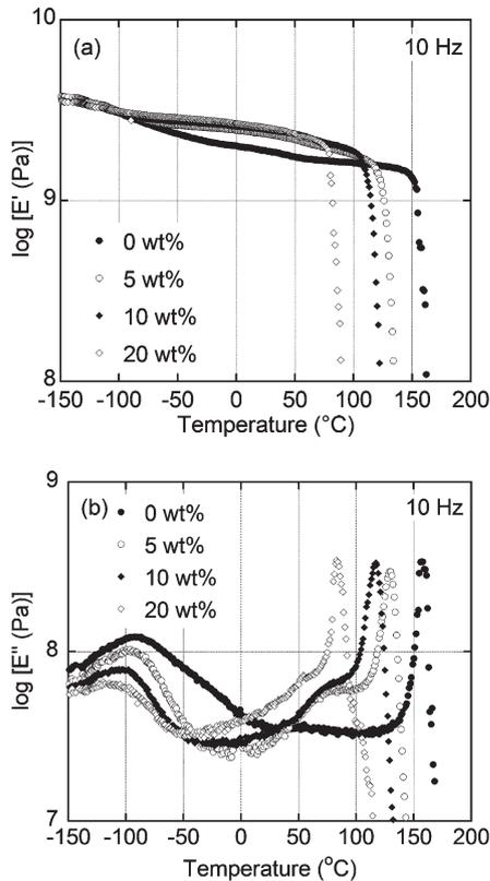
Fig. 1. Temperature dependence of (a) tensile storage modulus  $E'$  and (b) loss modulus  $E''$  at 10 Hz for (closed circles) PC, (open circles) PC/*p*-tPh (5 wt%), (closed diamonds) PC/*p*-tPh (10 wt%), and (open diamonds) PC/*p*-tPh (20 wt%).
