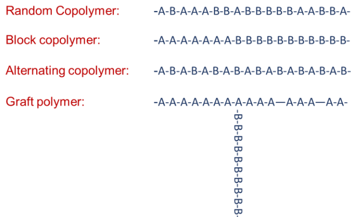
Figure 1.1 Schematic Representation of classification of polymers is based on the arrangement of the repeating units in a copolymer.
