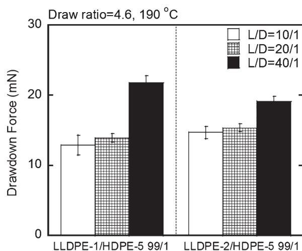
Fig.4. Drawdown force of the blends evaluated using various dies at a draw ratio of 4.6; (left) LLDPE-1/HDPE-5 (99/1) and (right) LLDPE-2/HDPE-5 (99/1). The extrusion was carried out at 190 °C.
