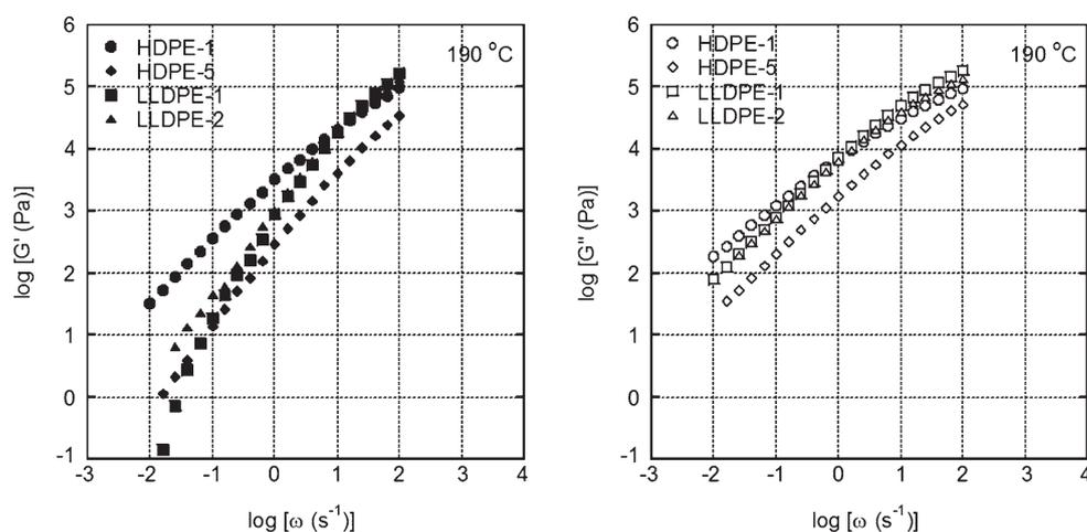
Fig. 1. Angular frequency dependence of oscillatory shear moduli such as storage modulus  $G'$  (left) and loss modulus  $G''$  (right) for HDPE-1 (circles), HDPE-5 (diamonds), LLDPE-1 (squares) and LLDPE-2 (triangles) at 190 °C.
