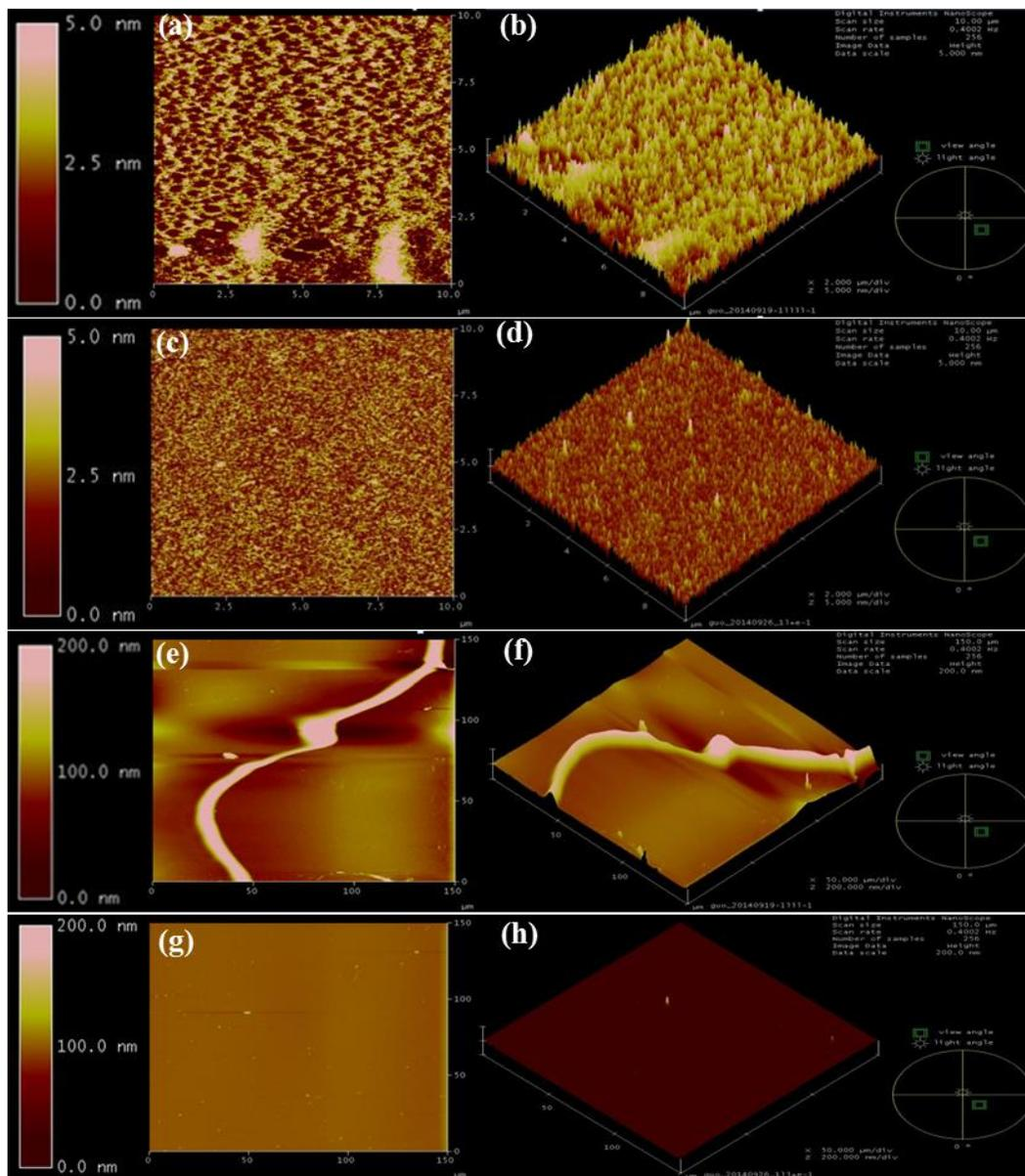
**Figure 4.** Tapping mode of atomic force microscope (AFM) images of Nafion thin film at the area without boundaries: (a, b) air vapor treated Nafion thin film with the surface of cell-like cavities and unevenness; (c, d) ethanol vapor treated Nafion thin film with a smoother and more uniform surface morphology; (e, f) air vapor treated Nafion thin film with a high thick boundary; and (g, h) ethanol vapor treated Nafion thin film with no boundaries in the film.
