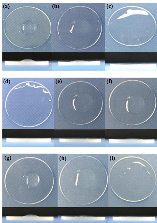
**Figure 2.** Top and side views (a, b, c) respectively depict 10 μL of sessile water droplet on substrates A, B, and C. In contrast, 10 μL of ink A dropped respectively on substrates A, B, and C (d, e, f) exhibited reverse wettability compared with the water droplet on the same substrate. 1020 μL of solvent itself dropped respectively on substrates A, B, and C (g, h, i).
