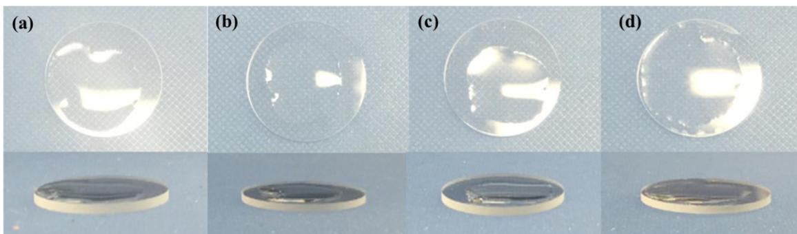
**Figure 6.** Hydrophilicity check (20 $\mu$ L of water drop) for the Nafion ultra-thin film: (a) as-prepared, (b) after ethanol vapor treatment, (c) after conductivity measurements under humidified conditions, and (d) after repeated ethanol vapor treatment.
