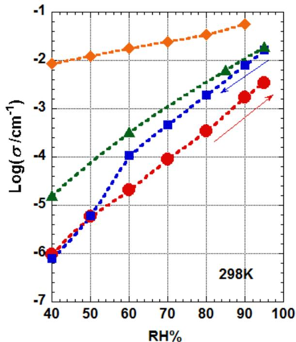
**Figure 5.** Relative humidity dependence of proton conductivity for the Nafion ultra-thin films: (●) 7 nm thick film treated by ethanol vapor, (■) 7 nm thick film by the second ethanol vapor treatment after the first conductivity measurement under humidified condition, (▲) 10-nm-thick Nafion thin film reported by Modestino *et al.*,<sup>37</sup> and (◆) Nafion 117 bulk membrane.<sup>43</sup>
