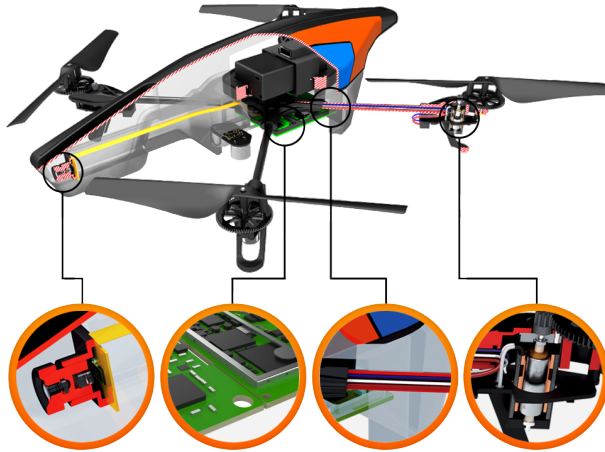
Figure 3.1: Aerial platform: Our aerial platform is AR.Drone , which is commercially available low cost platform.
