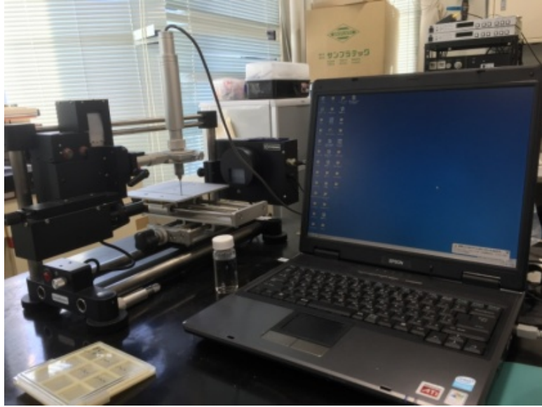
Figure 2-12. Surface energy measurement system.
