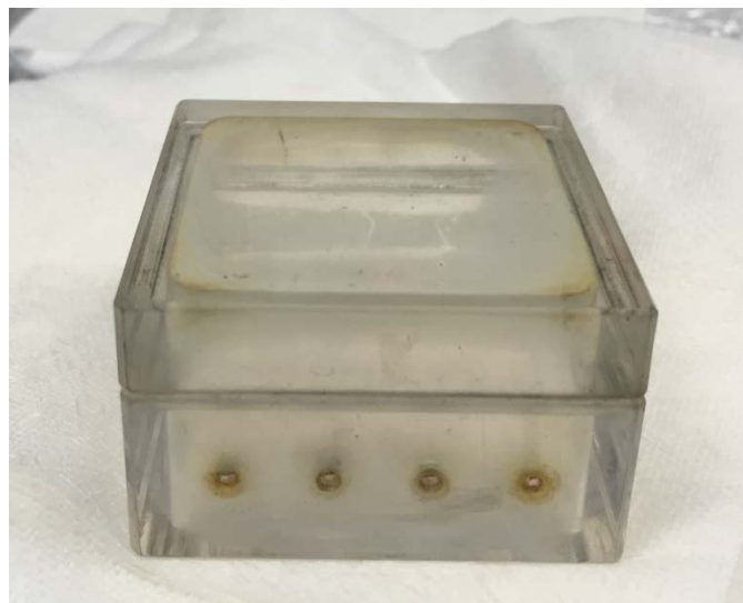
Figure 4-1. Picture of quartz box for thermal treatment of MoS 2 .
