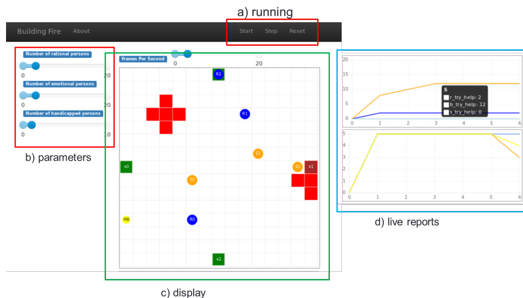
Figure 7-7 Simple UI presents the display of the live simulation that a learner can observe. Parts a and b, red colored rectangles, are allowed a learner to interact with. Part a. is a controller for running the simulation. It can control start/stop running, run step-by-step, and reset the simulation. Part b. is parameter settings. In this simple UI shows only number of each type of agent. Part c., green-colored rectangle, presents the movement of components in the simulation. The rectangles represent structures and incidents such as exits and fires. While the circles represent simulated agents. The red, green and brown colored rectangles present the fire, exit, and burnt exit, respectively. The burnt exit is the exit that covered with fire. It is broken and cannot be used for escape anymore. The blue, orange and yellow colored circles represent the rational, emotional, and handicapped agents, respectively. Part d., light blue colored rectangle, presents the live report about number of survivors, deaths, and other factors presented in Table 7-4. In the actual UI, the live reports is presented beneath part c.
