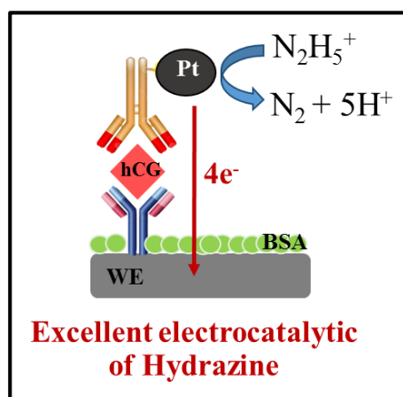
Figure 39. Schematic illustration of the electrocatalysis of hydrazine by PtNPs
