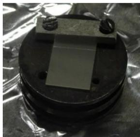
Figure 3.1.3.1. Introduce the TiO<sub>2</sub> (320) sample on a sample holder.
