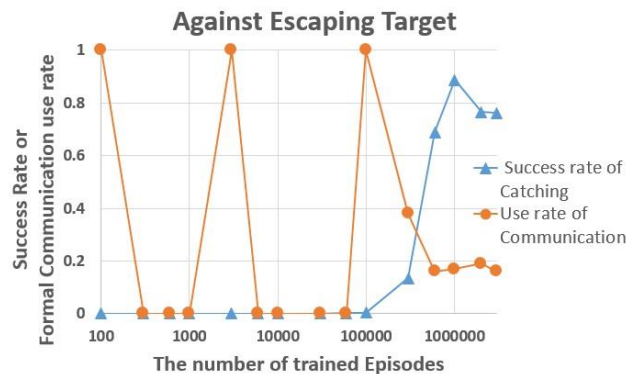
Fig. 6. Success rate and use rate of the communication function while chasing the escaping target. Eventually, agents began to avoid using the communication function in all but 20% of episodes.
