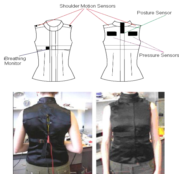
Figure 2.22: An example of smart health monitoring clothes – pressure sensors based breath monitoring
