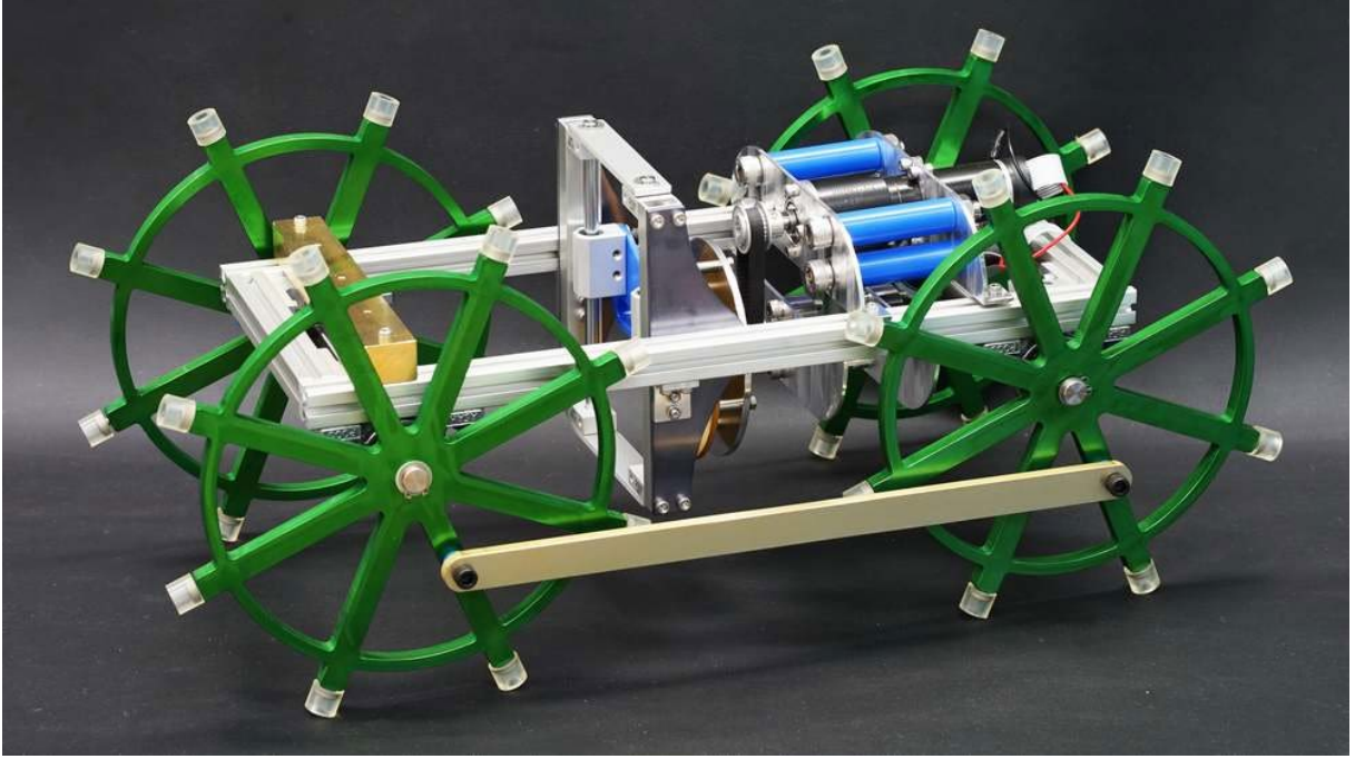
Figure 3.1: Experimental machine of combined rimless wheel with an active wobbling mass
