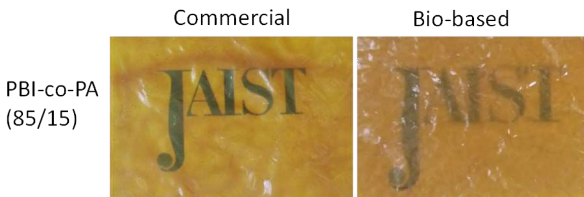
Figure 3.11 PBI-co-PA (85/15) copolymer films obtained both in commercial and bio-based methods
