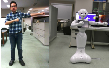
Fig. 4. Human pose and the mapped one on Pepper robot
