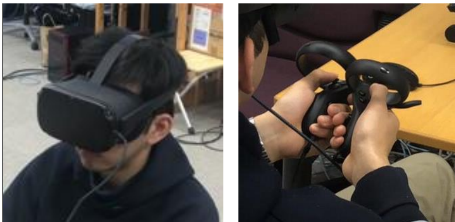
Figure 13. Participants use Oculus Quest HMD (Left) and Oculus touch controller (Right) to move in the VR environment.
