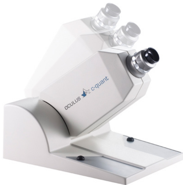
Figure 2.3: C-Quant device to measure light scattering [24]
