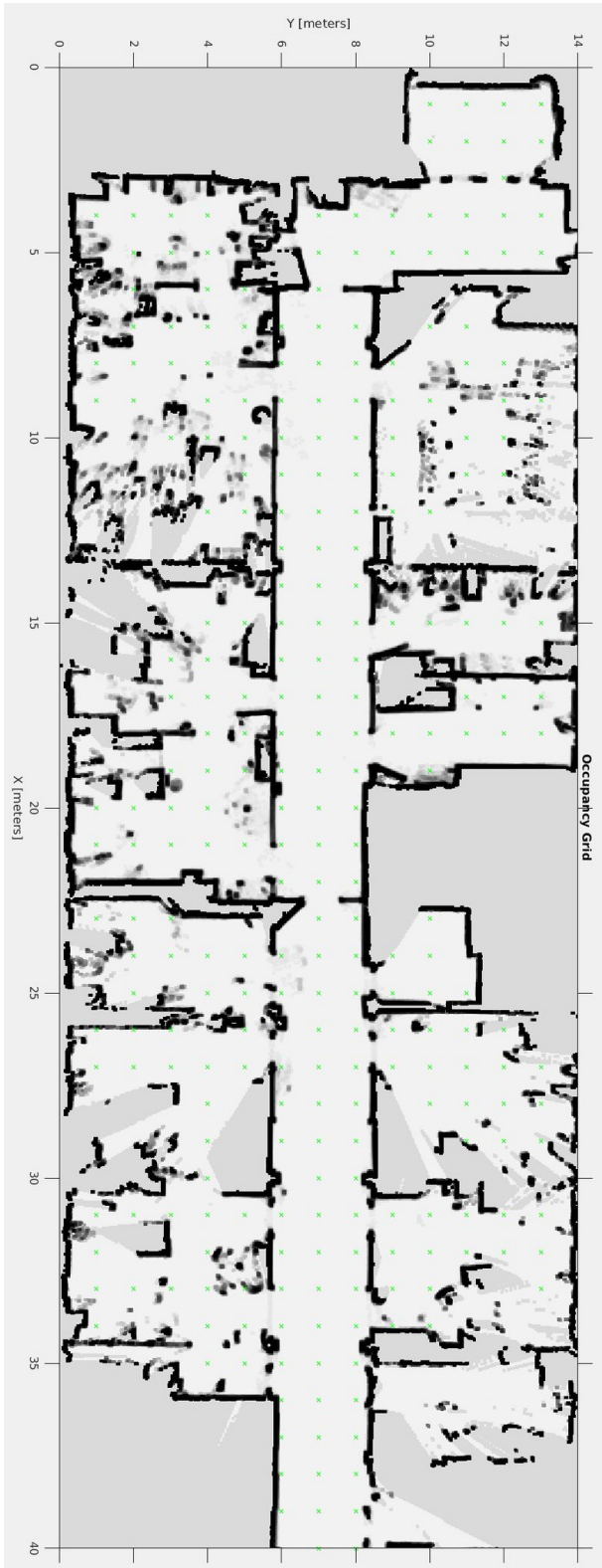
Figure 5.23: Frontier cells are generated on free space by removing those frontier cells which are out of bound.
