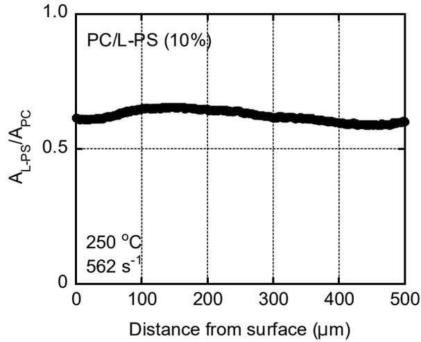
Figure 8 Distribution of  $A_{L-PS}/A_{PC}$  in the cross-section of extruded PC/L-PS (10%, 250 °C, and 562 s<sup>-1</sup>) strand
