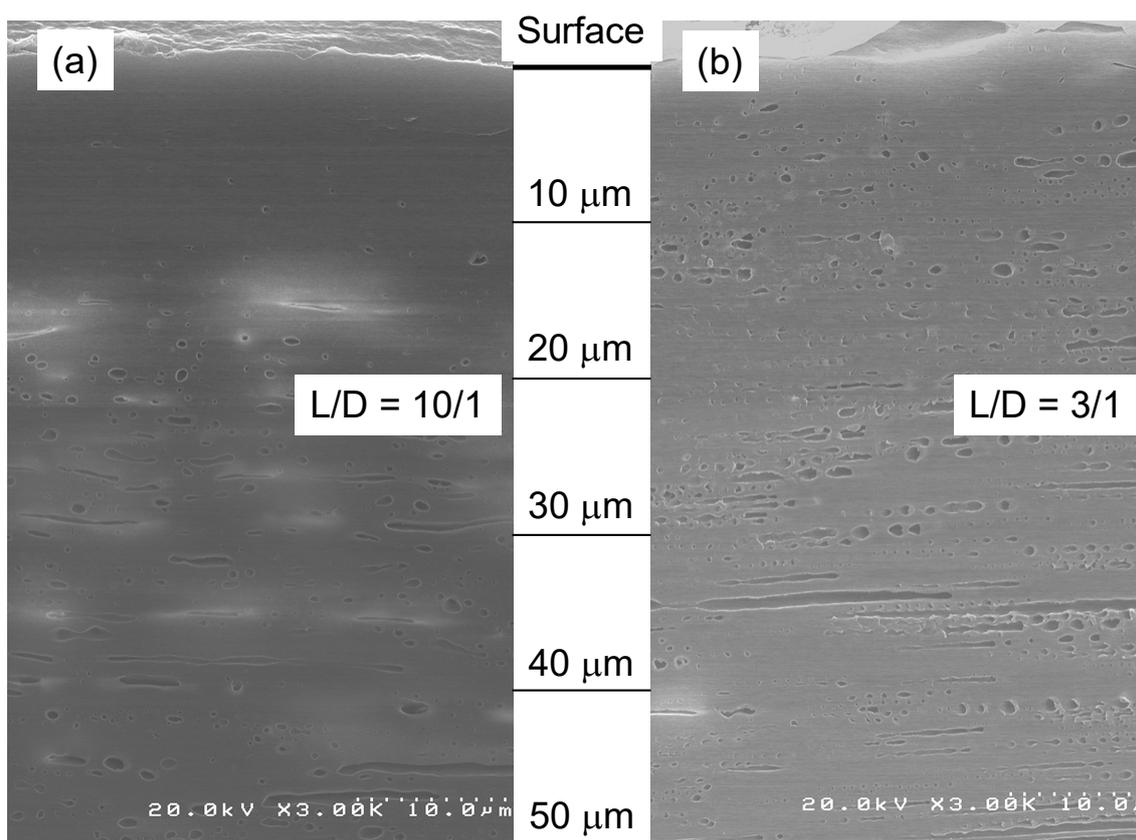
Figure 11 SEM images of the surface region in the cross-section for the PC/L-PS (10%) strand extruded from a circular die with  $L/D$  ratios of (a) 10/1 (mm) and (b) 3/1 (mm) at 250  $^{\circ}\text{C}$  and 562  $\text{s}^{-1}$ . Both samples were quenched by iced water immediately
