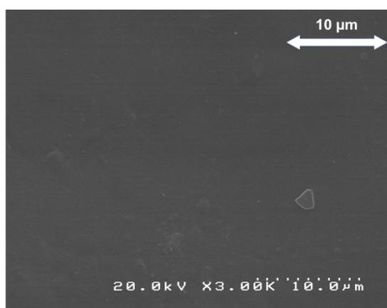
Figure 12 SEM image of the strand surface for PC/L-PS (10%) extruded from a die with  $L/D = 10/1$  at 250 °C and  $562 \text{ s}^{-1}$
