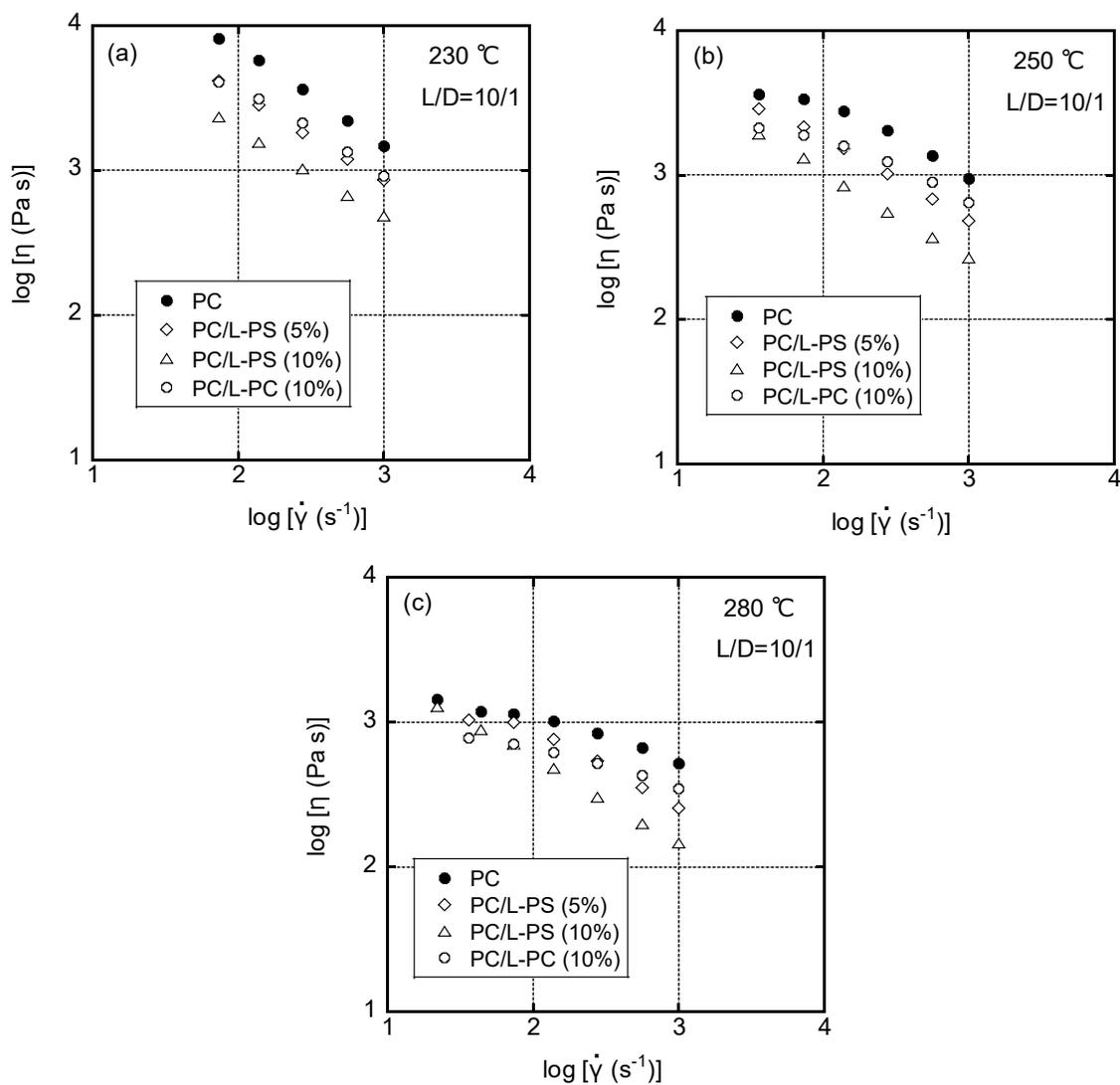
Figure 3 Flow curves at capillary extrusion for PC, PC/L-PS (5%), PC/L-PS (10%), and PC/L-PC (10%) at (a) 230 °C, (b) 250 °C, and (c) 280 °C
