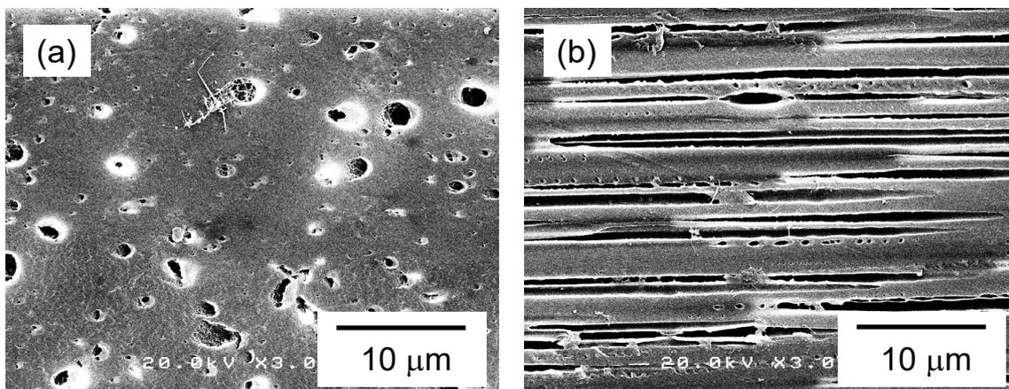
Figure 10 SEM images of (a) surface and (b) core regions in the cross-section for the PC/L-PS (10%) strand extruded from a die with  $L/D = 10/1$  at  $250\text{ }^{\circ}\text{C}$  and  $562\text{ s}^{-1}$
