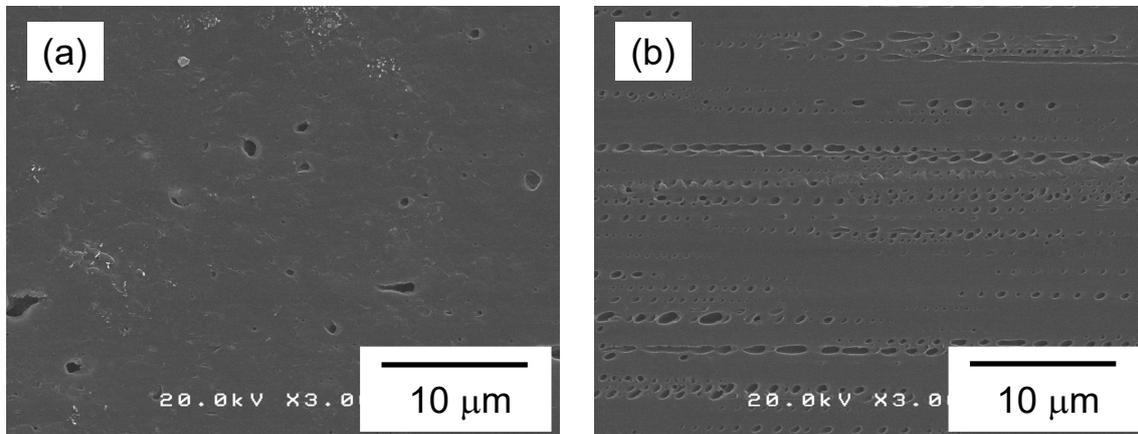
Figure 9 SEM images of (a) surface and (b) core regions in the cross-section for the PC/L-PS (5%) strand extruded from a die with  $L/D = 10/1$  at  $250\text{ }^{\circ}\text{C}$  and  $562\text{ s}^{-1}$
