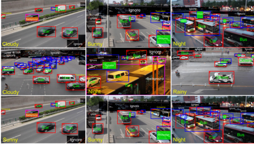
Figure 1.4: Example of detection-based approaches, where blue and red bounding boxes are represented as vehicle locations in the images [88].
