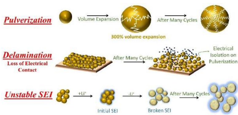
Figure 4: Drawbacks associated with Si anodes
