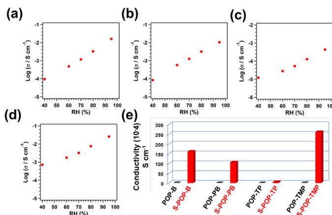
**Fig. 3.** Proton conductivities of (a) S-POP-B, (b) S-POP-BP, (c) S-POP-TP, and (d) S-POP-TPM measured at 25 °C under different RH. (e) Proton conductivities of POPs and S-POPs under 95% RH and 25 °C.
