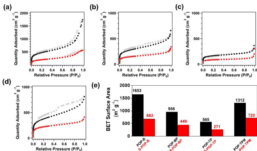
**Fig. 2.** Nitrogen sorption isotherms of (a) POP-B and S-POP-B, (b) POP-BP and S-POP-BP, (c) POP-TP and S-POP-TP, and (d) POP-TPM and S-POP-TPM measured at 77 K (●, adsorption; ○, desorption; black curves for POP and red curves for S-POP). (e) Comparison of BET surface area of POPs and S-POPs.
