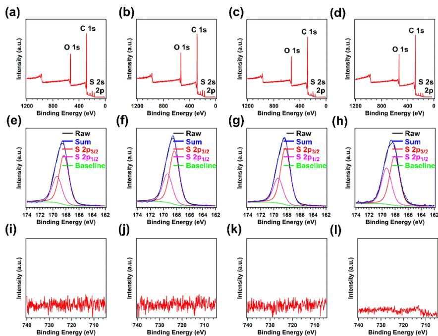
**Fig. 1.** X-ray photoelectron spectroscopy (XPS) spectra of (a) S-POP-B, (b) S-POP-BP, (c) S-POP-TP, and (d) S-POP-TPM. XPS analysis of S of (e) S-POP-B, (f) S-POP-BP, (g) S-POP-TP, and (h) S-POP-TPM. XPS analysis of Fe of (i) S-POP-B, (j) S-POP-BP, (k) S-POP-TP, and (l) S-POP-TPM.
