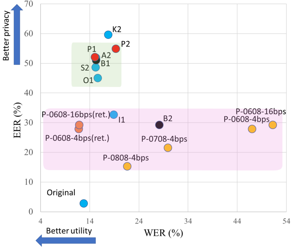
Figure 6.14: Mean WER versus mean EER over VCTK dataset in (o-a) scenario obtained from various systems proposed in Voice Privacy Challenge 2020. Black dot refers to results obtained by the baseline system. Red dot refers to results obtained by methods in [76]. Yellow and orange dots refer to results obtained by proposed methods. Blue dot refers to results obtained by other systems proposed in Voice Privacy Challenge 2020. The dots in the green shaded area are methods based on a neural vocoder (mainly based on the primary baseline framework). The dots in the pink shaded area are methods based on the LP vocoder.
