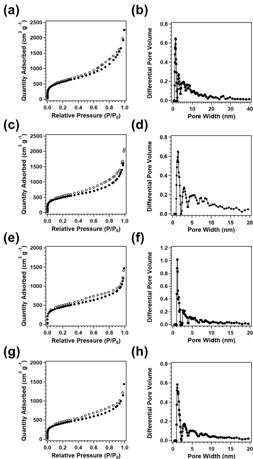
**Fig. 2.** Nitrogen sorption isotherms of (a) POP-BP, (c) i-POP-BP-BPTM-1, (e) i-POP-BP-BPTM-2, and (g) i-POP-BP-BPTM-3 measured at 77 K (●: adsorption, ○: desorption). Pore size distribution of (b) i-POP-BP, (d) i-POP-BP-BPTM-1, (f) i-POP-BP-BPTM-2, and (h) i-POP-BP-BPTM-3.
