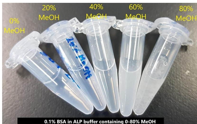
Figure 2.4.3.3 Methanol (MeOH) concentration (0-80% v/v) in the running buffer.
