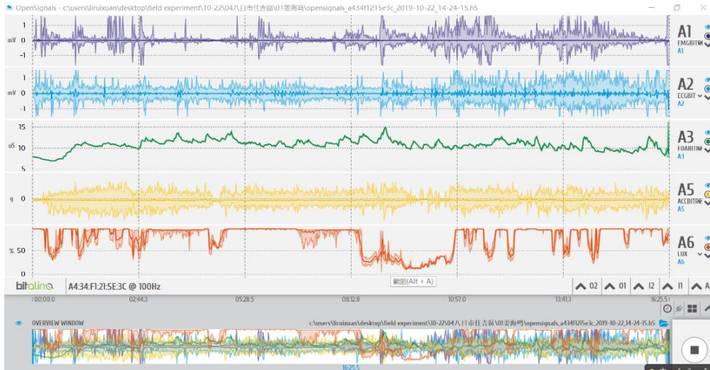
Figure 3.5 Physiological signals collected in space (A1: EMG signal; A2: ECG signal; A3: EDA signal) stored on a laptop through the supporting software OpenSignals_(r)evolution_win64.
