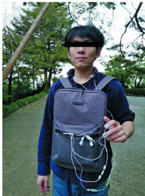
Figure 3.8 The participants wore a physiological signal feedback device (BITalino (r)evolution Plugged kit) and a head-wearing DV (Ordoro). They carried a GPS device (Nav-u NV-U73T, Sony) and a laptop computer as they walked through the space routes at a natural pace and constant speed. They could turn their heads to look at their surroundings. The computer automatically recorded the EDA, ECG, and EMG. The position where the electrodes of the physiological signal feedback instrument were pasted on the body: the two EDA electrodes were fixed on the first phalanx of the index and middle fingers; the ECG electrodes were fixed at the carotid arteries on both sides of the neck; the EMG electrodes were fixed on the inner side of the forearm of the arm.
