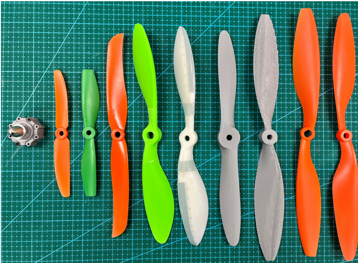
FIGURE 7.3: TomboHub universal design for assembly with various sizes propeller
