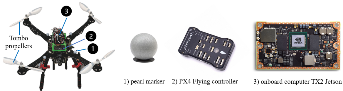
FIGURE 6.2: Main hardware of the experimental drone: Tombo propellers, pearl markers, a Px4 flying controller, and an onboard computer TX2 Jetson
