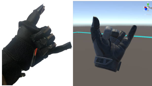
Figure 4.11: Static Gesture performed by VR Glove
