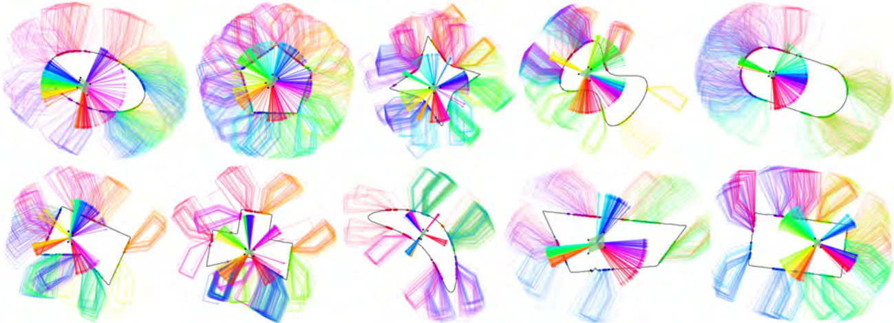
Fig. 16. Pushing directions that are available for each test object based on the intersected CoM region. Two-edge-contact pushing configurations are illustrated on the boundary of the object. The corresponding directions are illustrated on the centroid of the CoM region, using the same color.
