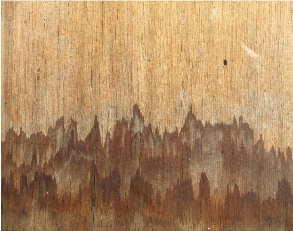
Figure 5-5: Hygroscopic nature of wood
