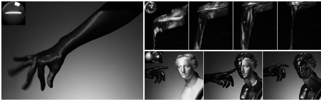
Fig. 3.3 Midas projection: markerless and modeled dynamic projection mapping for material representation [78].
