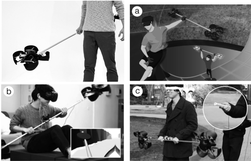
Fig. 5.2 LevioPole: Mid-air Haptic Interactions using Multirotor [134]
