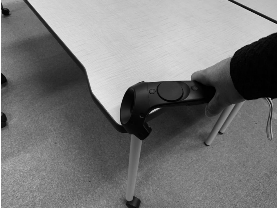
Fig. 3.12 Obtain coordinates of the play area using a Vive controller.
