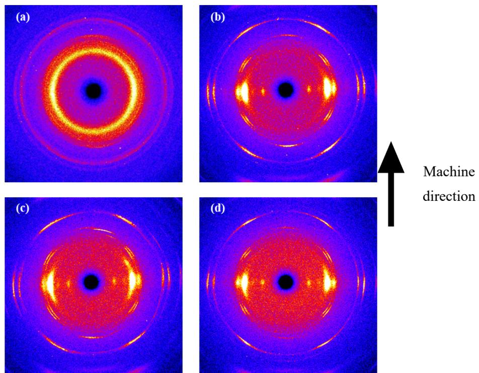
Figure 2-13 2D-WAXD images of PVA fiber stretched at 180 °C, 1.5mm/s (The machine direction is in the direction of the arrow).
