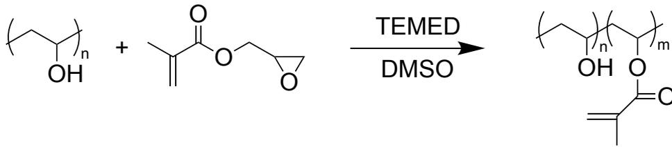
Figure 1-7 Synthesis of PVA methacrylate.
