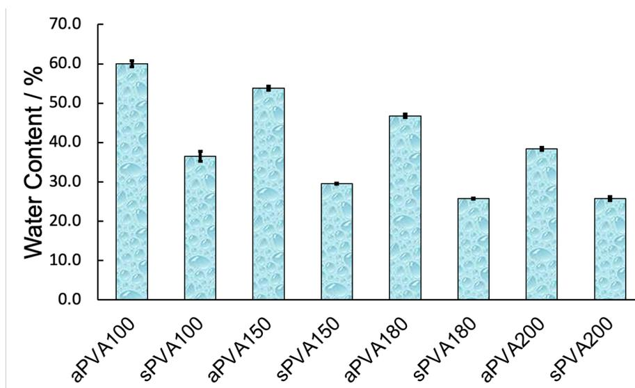
Figure 4-6 Water content of heat-treated aPVA-H and sPVA-H.
