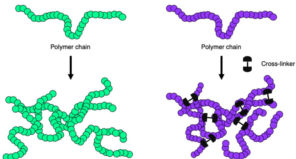
Figure 1-12 Schematic diagram of physical and chemical gels.
