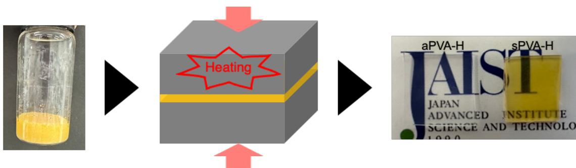
Figure 4-2 Gelation of PVA by hot press method.
