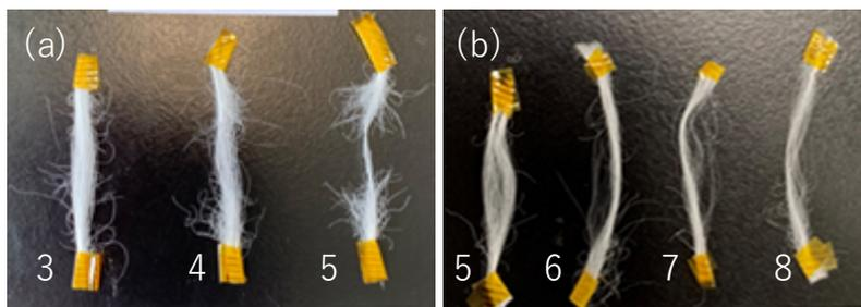
Figure 2-5 Heat-stretched of PVA fivers. (a) Pure PVA, (b) LiI PVA
