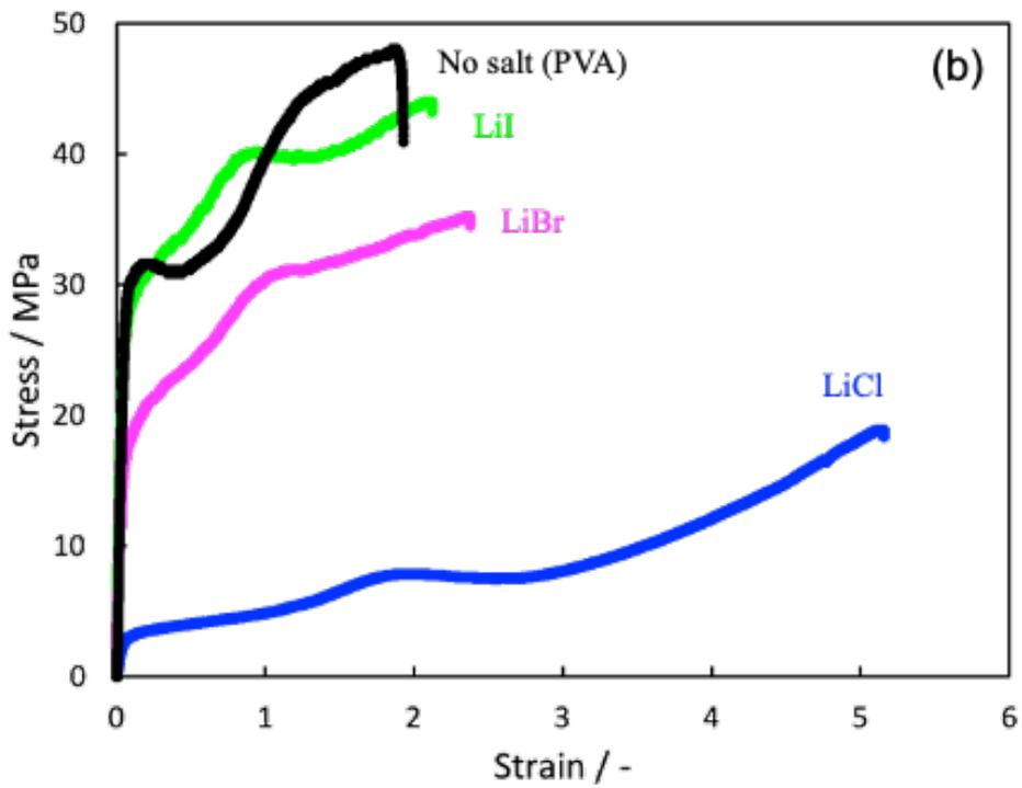
Figure 3-7 Stress-strain curves of PVA prepared by HP method with lithium salt.
