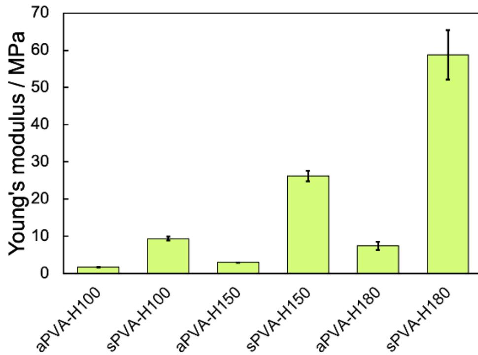
Figure 4-10 Young's modulus obtained by tensile testing.
