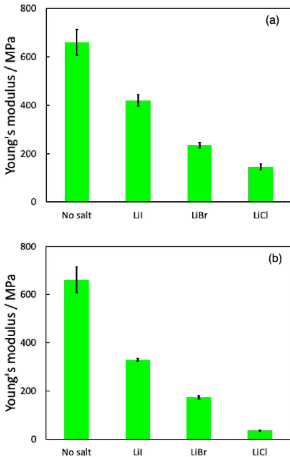
Figure 3-8 Young's modulus of PVA prepared by HP method with lithium salt.
