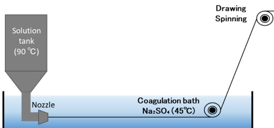
Figure 2-1 Schematic diagram of wet spinning machine.
