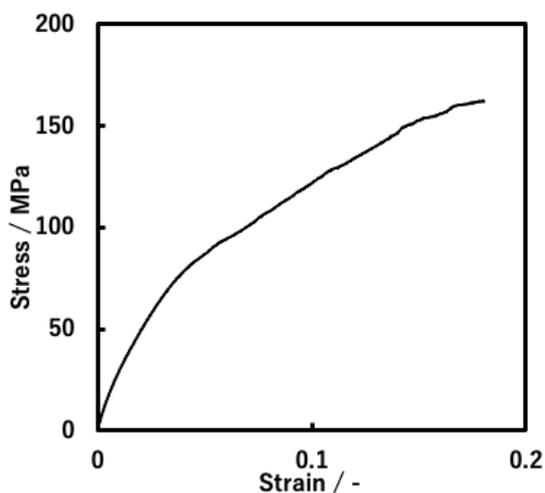
Figure 2-6 Stress-Strain curve of non-drawing fiber (PL4).
