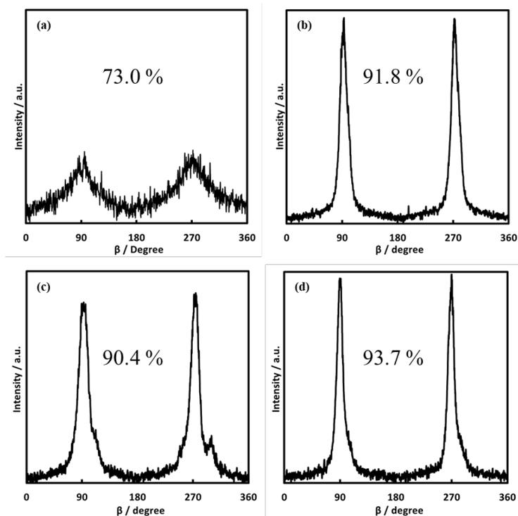
Figure 2-16 Azimuthal distribution in the (101) plane of PVA fibers stretched at 180 °C, 1.5mm/s.
