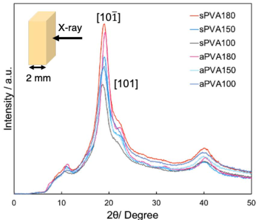
Figure 4-11  $2\theta$  profiles of aPVA-H and sPVA-H.
