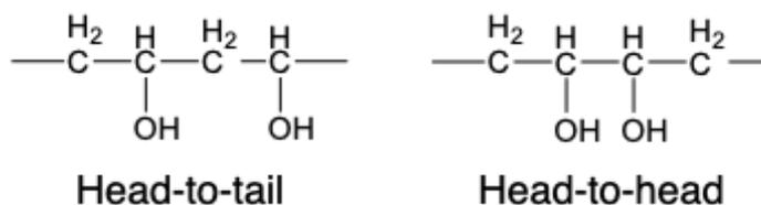
Figure 1-4 Head-to-head and head-to-tail structures of PVA.
