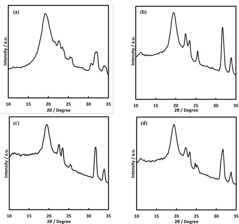
Figure 2-14  $2\theta$  profiles of PVA fibers stretched at 180 °C, 1.5mm/s.
