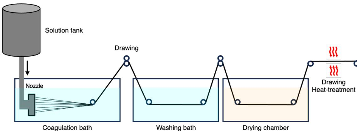
Figure 1-9 Wet spinning process for PVA fiber.
