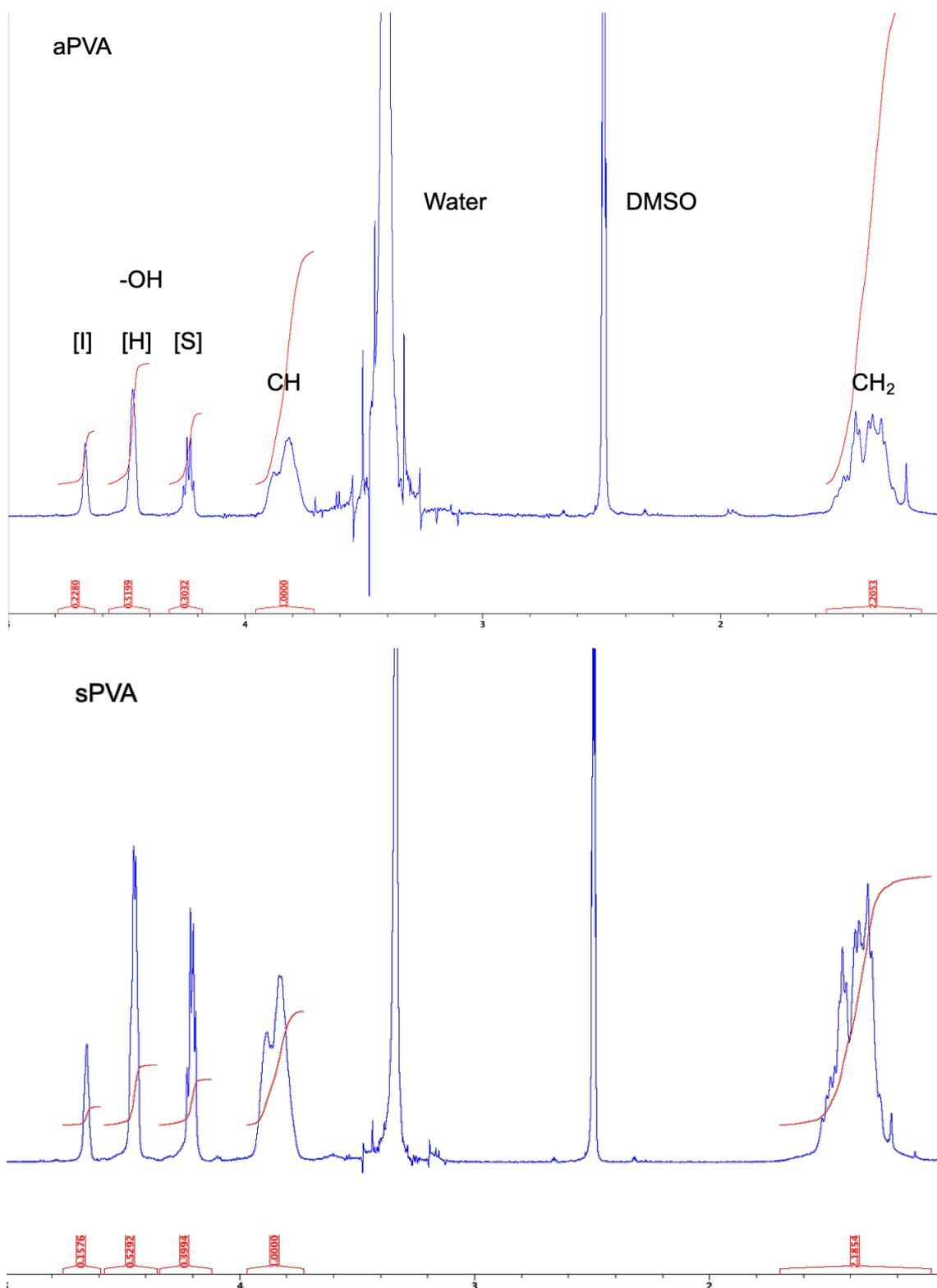
Figure 4-5 <sup>1</sup>H-NMR spectra of aPVA and sPVA.
