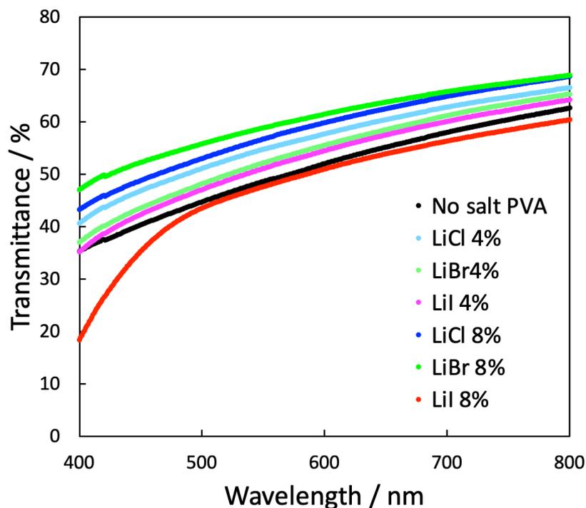
Figure 3-2 Light transmittance of PVAs.
