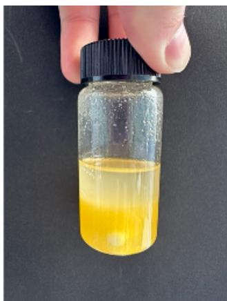
Figure 4-3 sPVA not dissolved in a mixture of DMSO and water.
