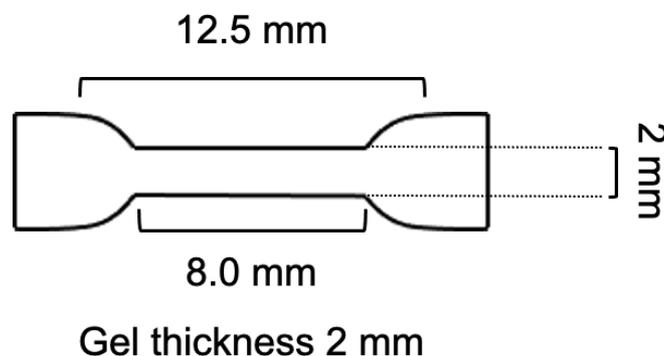
Figure 4-4 Shape of dumbbell-shaped specimen.
