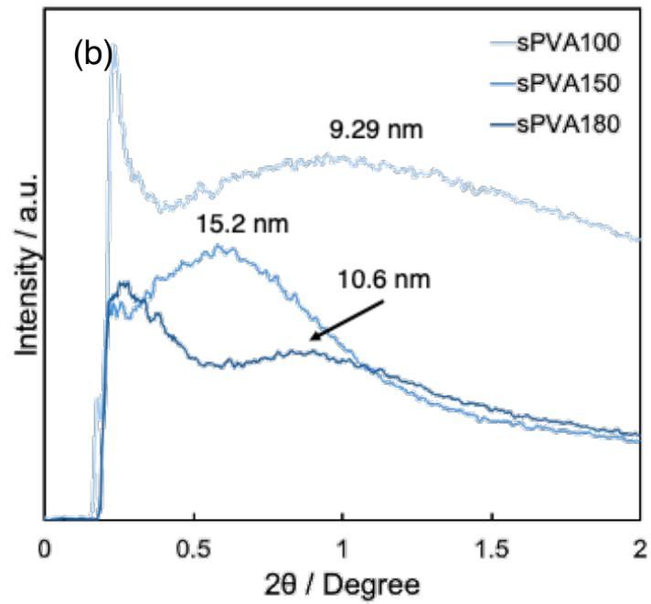
Figure 4-12 SAXS profiles of aPVA-H and sPVA-H.
