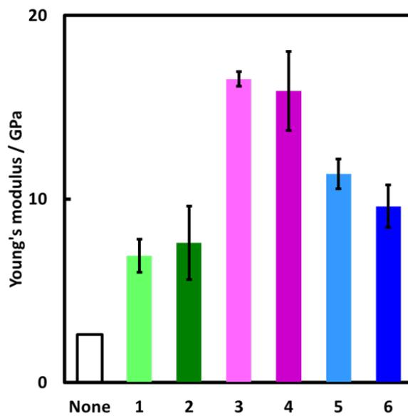
Figure 2-12 Comparison of young's modulus of fibers stretched at 180 °C, 1.0 mm/s and 1.5 mm/s.
