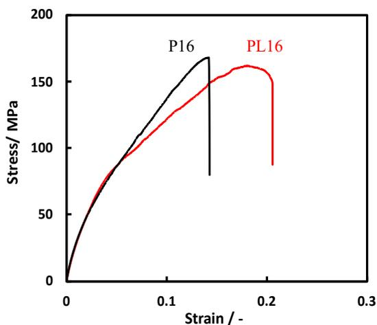
Figure 2-7 Stress-strain curves for P16 and P16 fibers.
