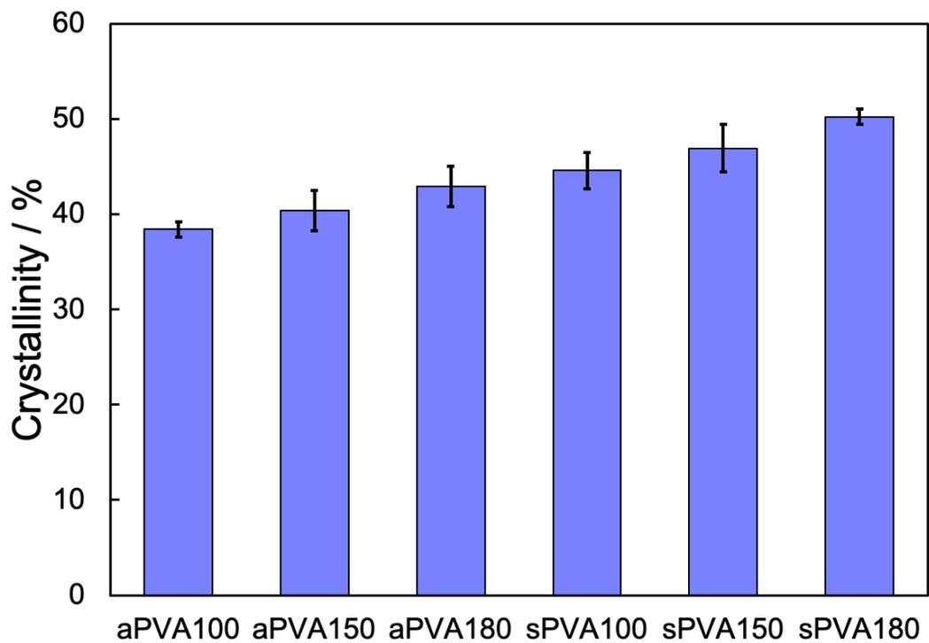
Figure 4-8 Comparison of crystallinity calculated from IR spectra.
