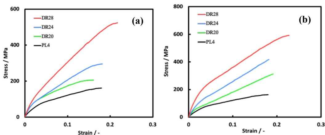
Figure 2-9 Stress-Strain curves of PVA fibers stretched at 180 °C, 1.0 mm/s. (a) Heat-treatment at 120 °C for one night, and (b) Heat-treatment at 150 °C 1 hour
