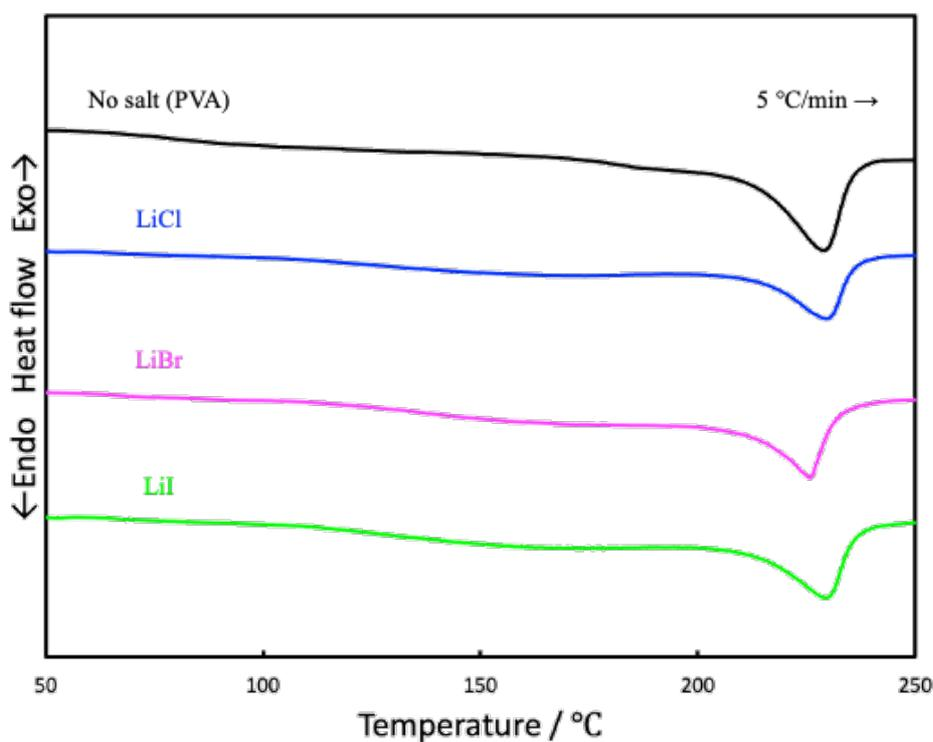
Figure 3-6 DSC heating curves of PVA after washing and desalting.
