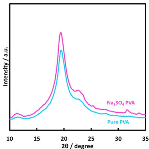
Figure 2-15  $2\theta$  profiles of Pure PVA film and PVA film with sodium sulfate.  $\text{Na}_2\text{SO}_4$  PVA film shows a characteristic peak between  $32^\circ$  and  $35^\circ$ , which is not seen in Pure PVA.
