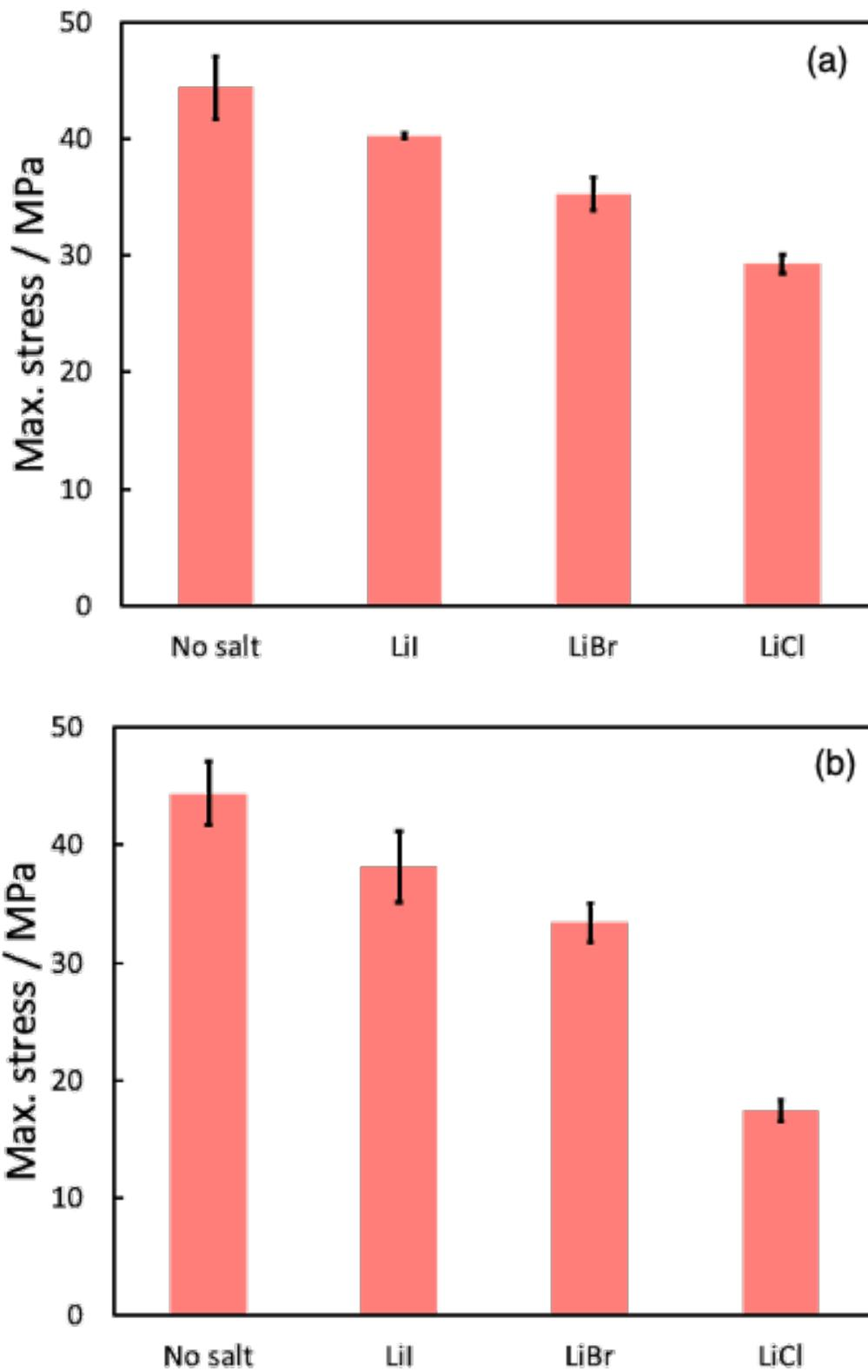
Figure 3-9 Maximum tensile stress of PVA prepared by HP method with lithium salt.
