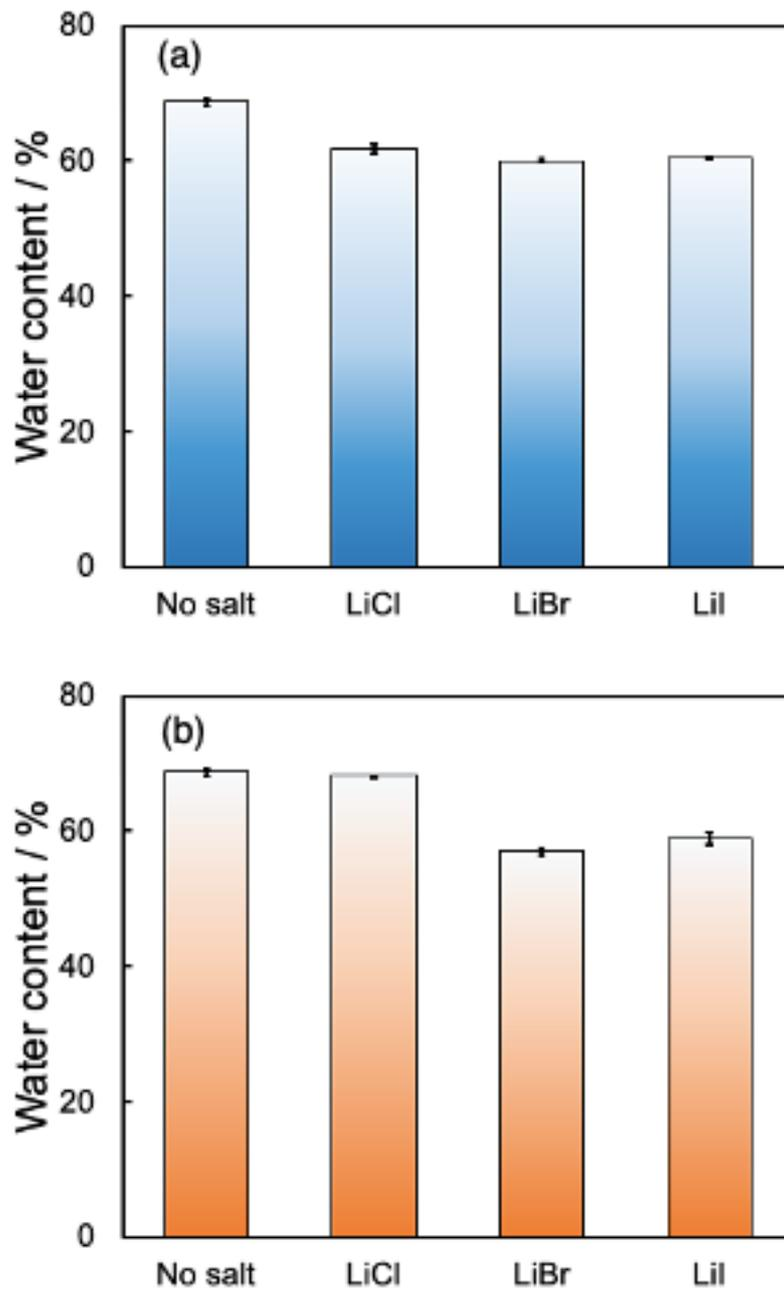
Figure 3-13 Water content of PVA prepared by the HP method with the addition of lithium salt.
