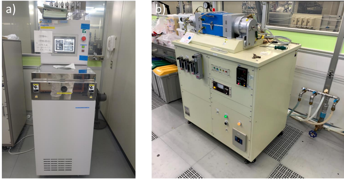
Figure 3.2 (a) Reactive Ion Etching machine. (b) Infrared furnace used during annealing.
