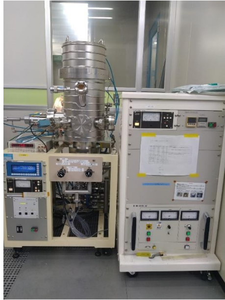
Figure 3.5 Electron beam thermal evaporator used during physical vapor deposition.
