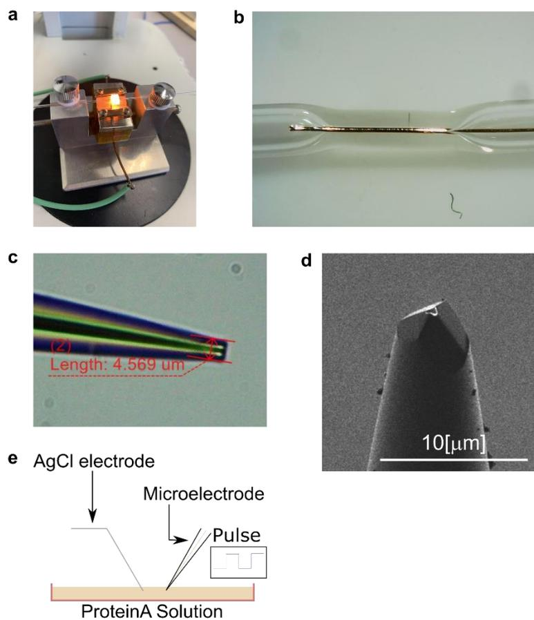
**Fig. 1.** Fabrication Process of Glass Microelectrodes. (a) Heated by the filament of the sealing machine, the gold is sealed inside the glass tube. (b) Sealed glass tube. (c) Glass tube immediately after pulling with a micropipette puller. (d) Tip of a glass tube electrode processed by the FIB system. Scale is 10[ $\mu\text{m}$ ]. (e) Schematic diagram of protein immobilization experiment.
