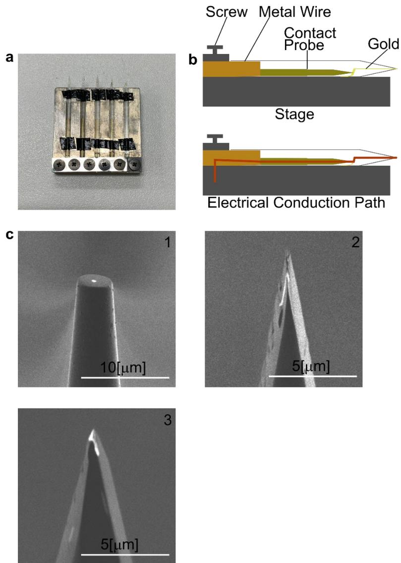
**Fig. 4.** Preparation for FIB processing and FIB processing. (a) 30[mm] square size stage for FIB processing. (b) Side view of the stage (upper). Red lines indicate conduction paths (lower). (c) FIB process flow. (1) Cut horizontally to expose the gold. (2) Cut the left and right sides. (3) Cut again twice at different angles. The pyramidal shape is obtained.
