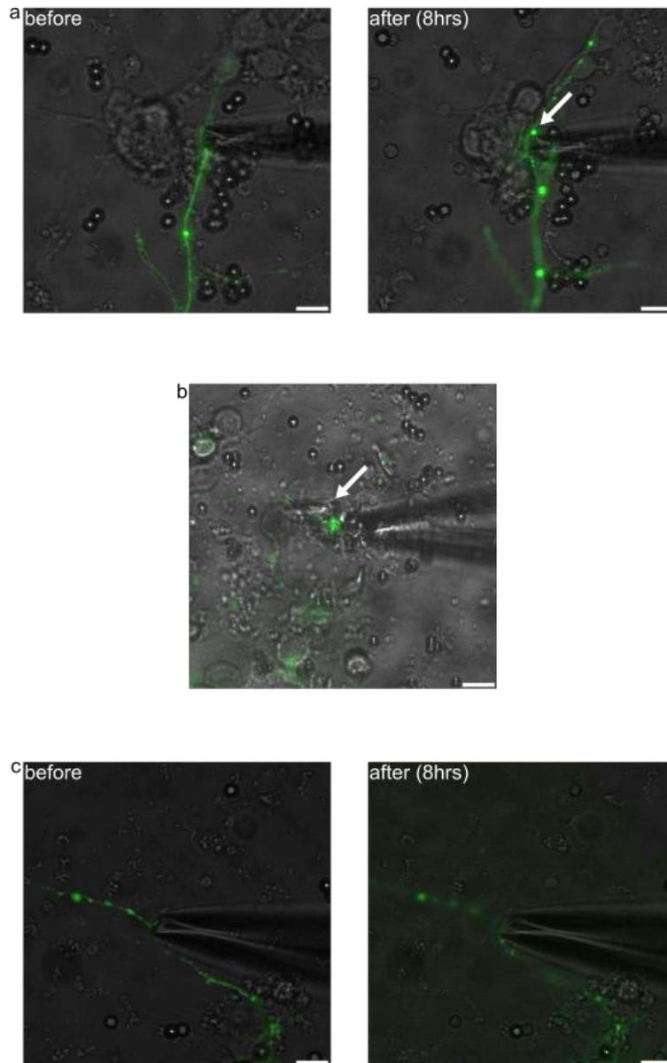
**Fig. 6.** Typical failure of an experiment using glass microelectrodes. (a) Rab3 (modified with fluorescent protein) accumulated on the non-gold tip of the electrode. (b) The tip of the electrode touched the bottom and was broken. (c) The slight movement of the electrode during 8 hours of incubation prevents it from contacting the axon (out of focus). Bars = 10  $\mu\text{m}$ .
