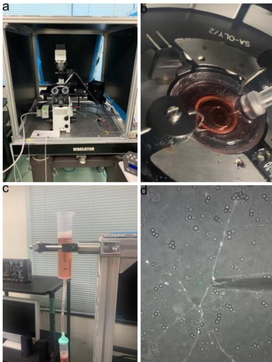
**Fig. 1.** Appearance of the experimental environment. (a) The area around the microscope, including the irrigation system, manipulators for electrode manipulation, and wiring for heaters. (b) A glass plate containing a Chick neuron culture is placed above the microscope lens. An electrode is approaching from the right. (c) L15 culture medium being pumped by the perfusion system. (d) Typical neuron in this environment. The electrode is in contact with the axon.
