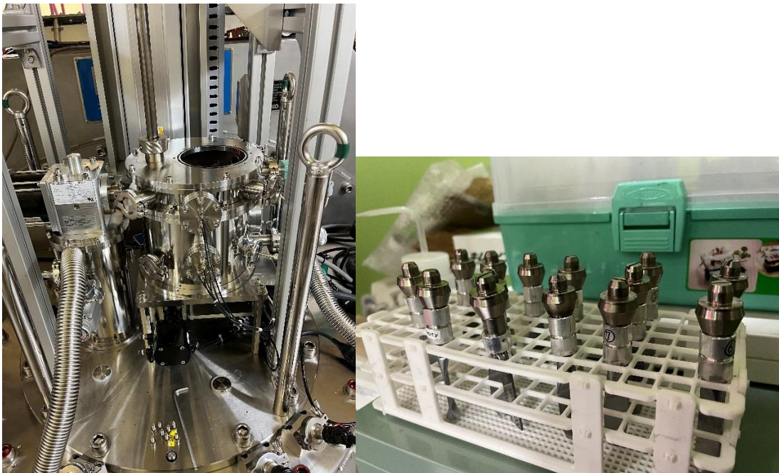
Figure10 NOVA sample insertion port used for measurement and image of the measured sample
