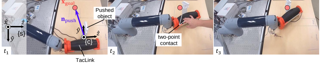
(a) Video stills of contact-based object pushing experiment with the possible occurrence of two-point contact.
