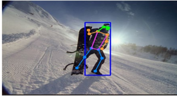
Figure 3.5 Key points regression of the human body by YOLOPose[12]
