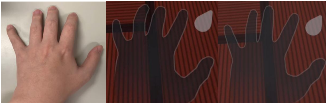
Figure 1.6: Jitter results in inaccuracies in the representation of the virtual model's position, leading to difficulties in interaction. The position of the virtual objects in the image appears blurred and unclear due to jitter, preventing real-time and accurate representation of their locations.
